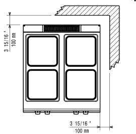
EI = Electrical connection EQ = Equipotential screw
