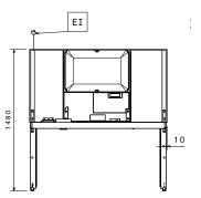
EI = Electrical connectionRI = Refrigerant InletRO = Refrigerant Outlet
